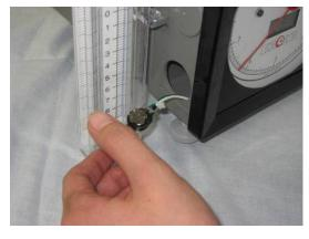
To take away a battery from the box. (to open metal hook to outside is easier)
