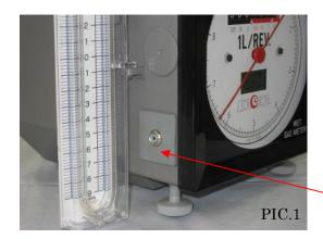
There is a cap (rubber) for battery box at the left side of front panel.
