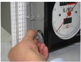
Attach from the lower part and confirm back to the normal, which the inside catch of cap is held to gas meter body.
